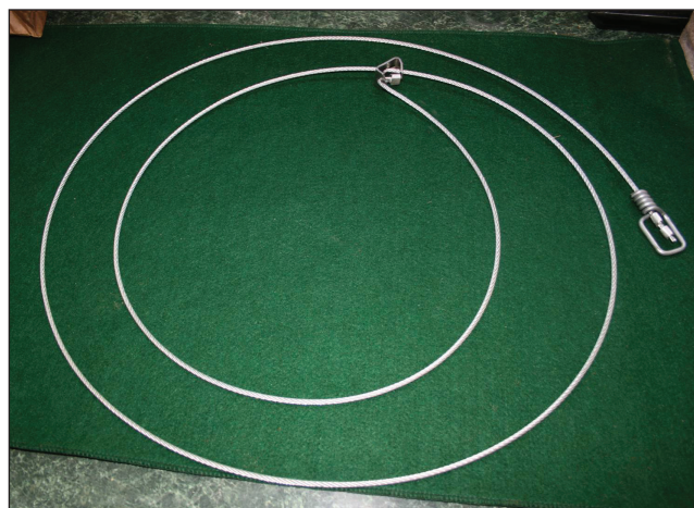
Figure 18. A complete 1/8-inch cable snare with a lock and end swivel for capturing feral hogs. Photo by James C. Cathey, Texas AgriLife Extension Service.
