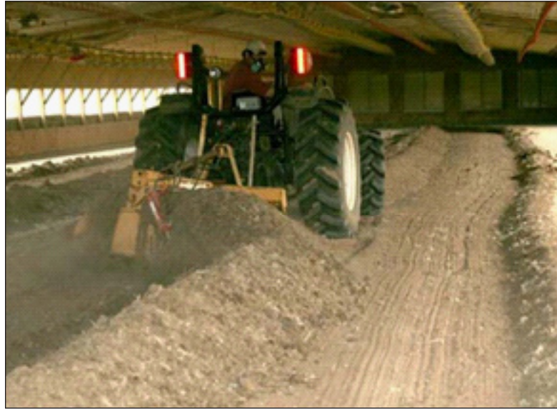
Figure 19. Windrows are formed inside a broiler production house. Photo by Craig Coufal, Texas AgriLife Extension Service.
