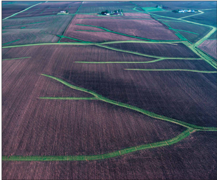
Figure 9. Grassed waterways carry runoff from fields helping prevent erosion and protect water quality. Photo by Lynn Betts, URDA-NRCS.
